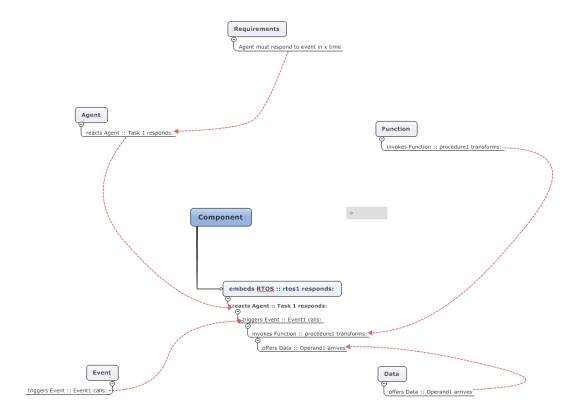
This is the nominal configuration in which there is a hardware processing node which has a Real Time Operating System (RTOS) on which are agents as tasks which are assigned functions that support dataflow triggered by events.
